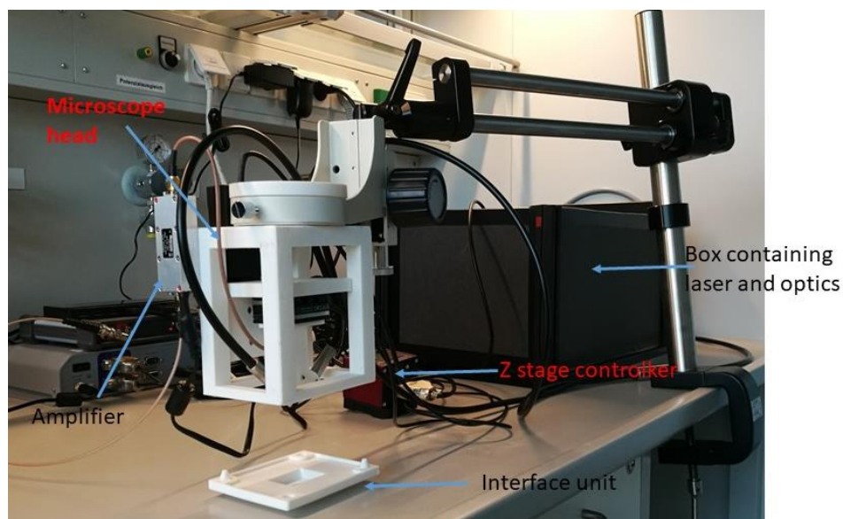
Figure 1: Perspective picture of the RSOM2. The black box contains the laser and the optics used to bring the laser pulses to the sample. Initially, an interface unit is attached to the sample. Afterwards the scanning head is attached to the interface unit. A small amount of water is introduced in the interface unit to ensure acoustic coupling between the tissue and the transducer.
